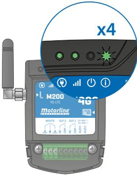
3 • Wait until the ACT LED starts flashing 4 times with 1 second interval;
