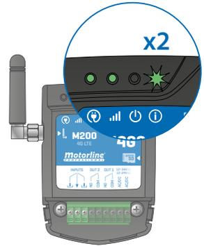
6 • Wait until the ACT LED starts flashing 2 times with 1 second interval;
