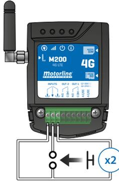
4 • Give two pulses simultaneously on the two inputs IN1 IN2 and GND;
